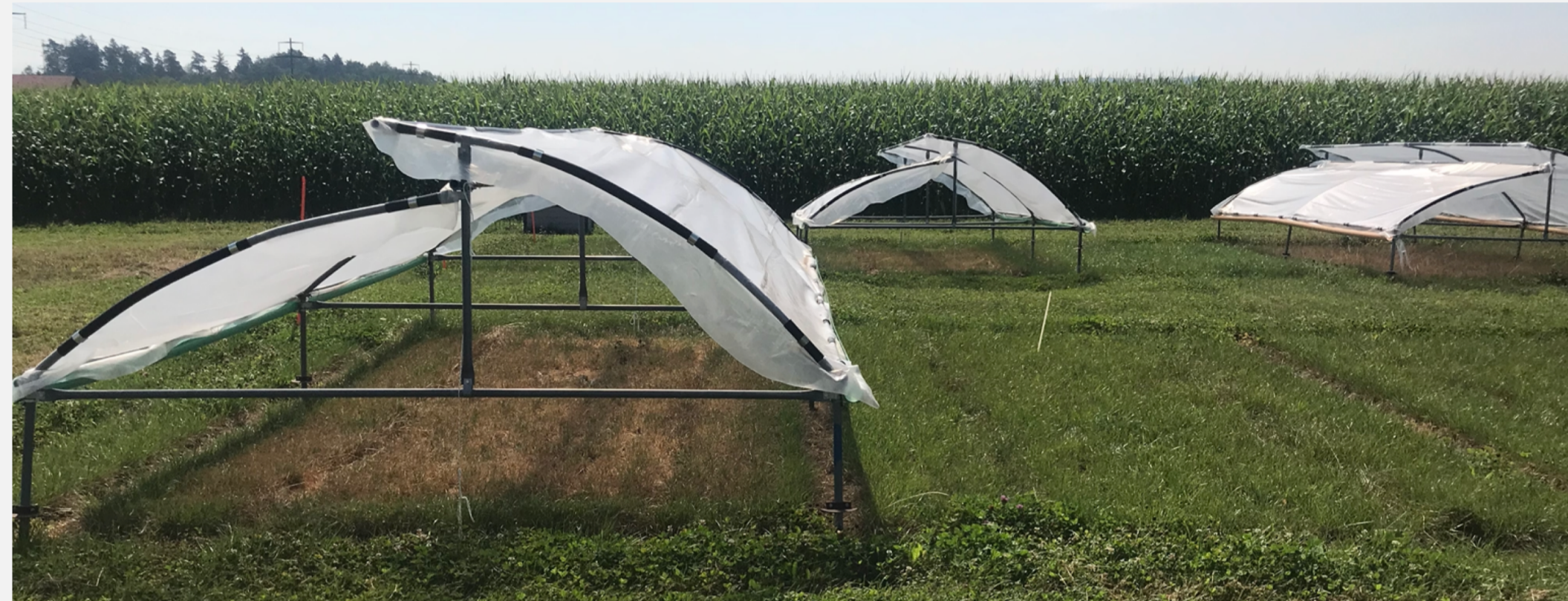
Fig. 1 Rainout shelters of 3 x 5 m were placed on used to simulate a severe summer drought of 2 months. Plots were re-wetted immediately after shelter removal.
